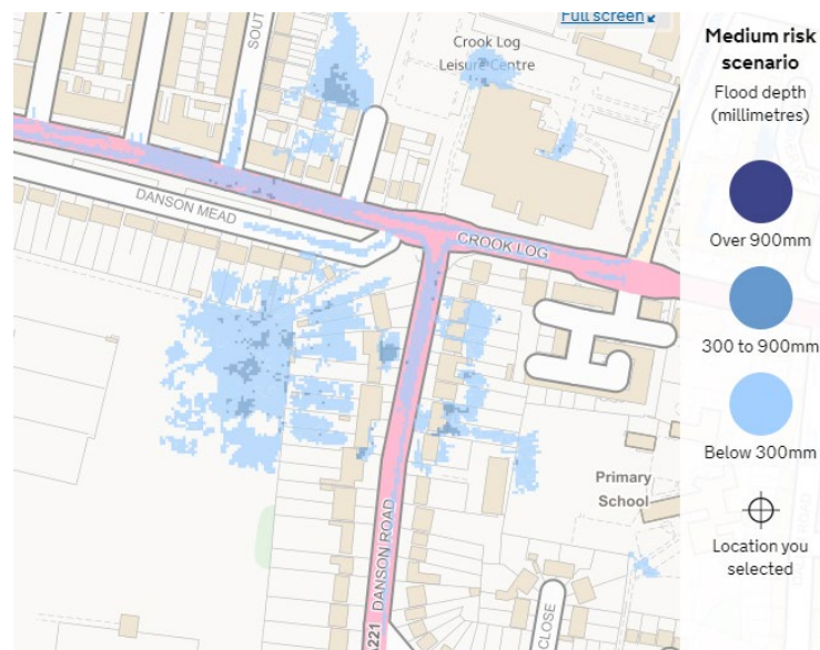
Figure 8: Localised Pluvial/Surface Water Flooding
