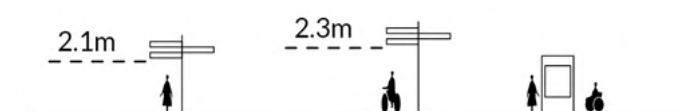
Fig.97 For safety, overhead signage should be 2.1m above a footway and 2.3m above a cycleway. Signs mounted on vertical surfaces should be at a suitable height to be read by all users.
