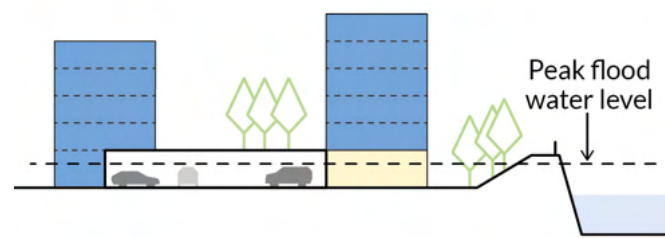
Fig.91 Habitable rooms in residential development within the fluvial flood zones, should be set 300m above the predicted 1 in 100 year plus climate change peak flood water level. Within the tidal flood zones, habitable rooms should be set above the predicted 1 in 200 year annual probability.
