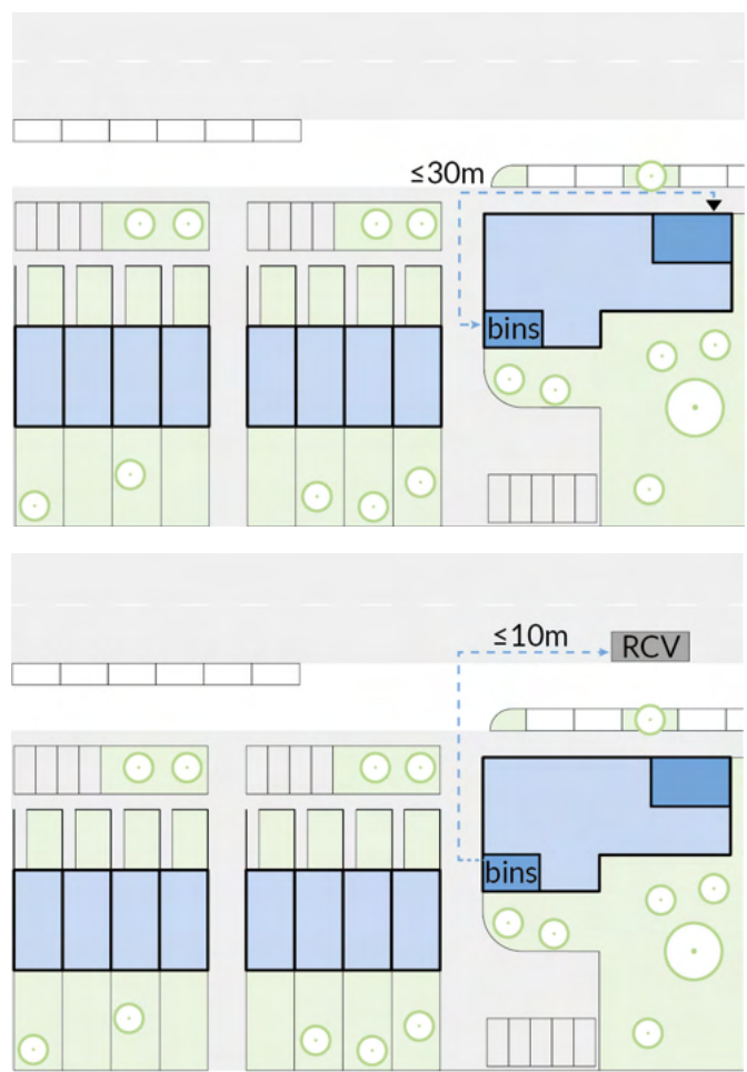
Fig.71 Waste facilities should be within 30m of any front door and no more than 10m from the collection point by Refuse Collection Vehicle (RCV), typically on the public highway.
