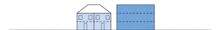
Fig.19 Pitched roofs can be considered a single storey when compared against flat roof buildings.
